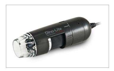
The Dino-Lite AM4116T connects directly to a VGA screen via a VGA (D-SUB) connector. It offers a high frame rate of up to 60fps at 640x480 resolution and has enhanced low light visibility so you can see clearly in any situation. The AM4116T is the ideal choice in situations, where real time images are vital. The LEDs can be switched on and off by using the MicroTouch sensor on the microscope.
