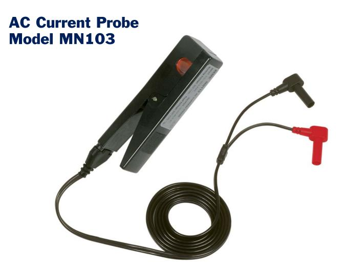
Small, compact and very tough, the Model MN103 is designed for measurements from 1mA to 100AAC. The "clothes pin" shape makes it ideal for use in tight areas, such as breaker panels, controller panels or outlets. It is an excellent companion to all DMMs.
