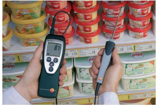
Inspecting the temperature of a refrigerated counter
