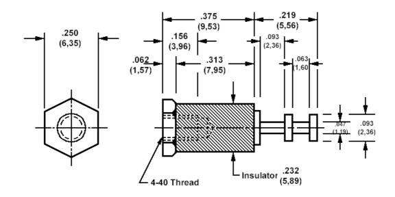
How to order code  $\underline{572\text{-}4826\text{-}01\text{-}\underline{YY}\text{-}\underline{16}}$  Basic Part No (YY = plating finish. See tables for options)
