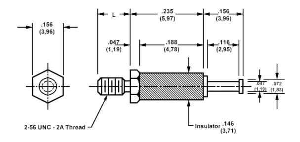
$\frac{572\text{-}4870\text{-}\text{XX}\text{-}\frac{YY}{16}}{\text{Basic Part No (XX = thread length, YY = plating finish. See tables for options)}}$
