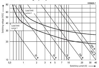
Load limit curve 1: arc extinguishes during transit time (CO contact). Load limit curve 2: safe shutdown, no stationary arc (NO contact). Load limit curves measured with low inductive resistors verified for 1000 switching events.
