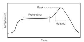
For soldering (Example : Sn/Pb)
