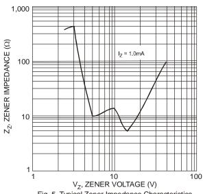
Fig. 5 Typical Zener Impedance Characteristics
