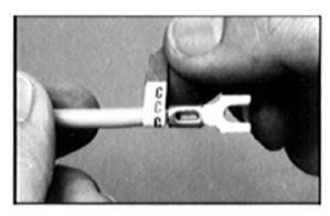
Pick up tab to remove marker from book. Complete the wrap, and flip the tab off.
