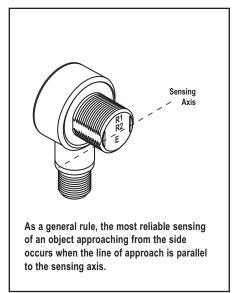
Figure 2. Fixed-field sensing axis
