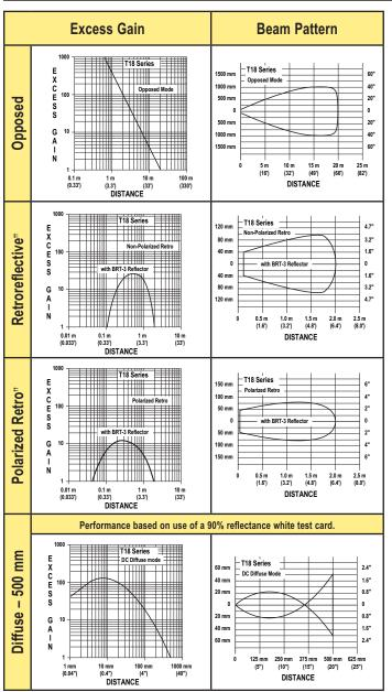
†† Performance based on use of a model BRT-3 retroreflector (3" diameter). Actual sensing range may be more or less than specified, depending on the efficiency and reflective area of the retroreflector used.
