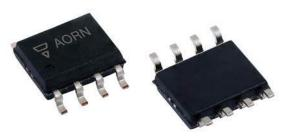
The AORN series features a narrow body (0.150") small outline SMT package. The network is constructed with a tantalum nitride resistor film on a high purity alumina substrate for improved ESD and moisture protection.
