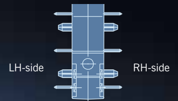
Side definition with terminals and location pins
