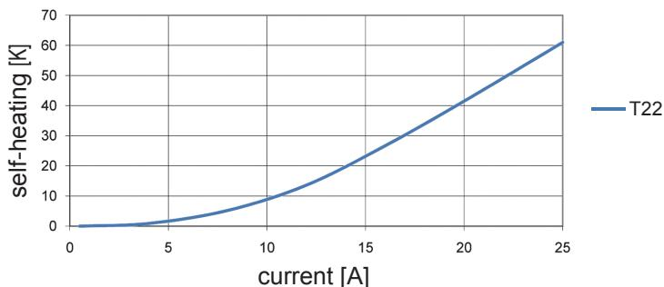
The characteristic curves are measured with a thermal control without any insulation in an oil bath.
