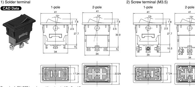
Remarks: 1. ON-OFF type does not have terminal No. 2 and 5  $\,$ 2. Dimensions of actuator: 1-pole: 12.6  $\times$  29, 2-pole: 17.4  $\times$  29
