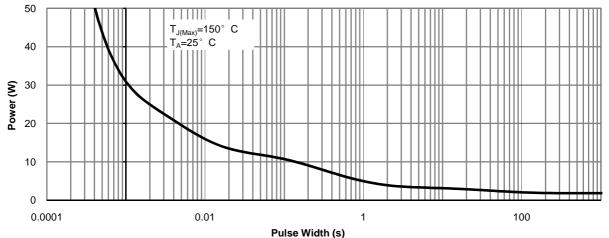
Figure 11: Single Pulse Power Rating Junction-to-Ambient (Note E)
