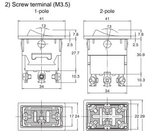
Remarks: 1. ON-OFF type does not have terminal no. 2 and 5. 2. Dimensions of actuator: 1-pole: 12.6 × 29, 2-pole: 17.4 × 29
