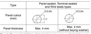
Remark: For panel installations of standard type, be use to use the back hex nut. ds\_62001\_0106\_en\_t15: 010314J
