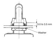
b. Enough screw pitch should be obtained being adjusted within 3 to 3.5mm (See figure above).
