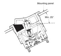
b. In case water inside the switch case may freeze, please install the switch vertically to avoid the water remain inside the switch.
