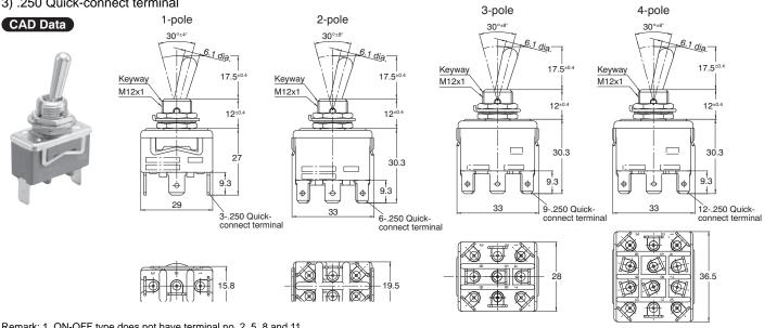
Remark: 1. ON-OFF type does not have terminal no. 2, 5, 8 and 11. 2. There is no through-hole on .250 Quick-connect terminals.
