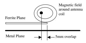
Optimum field distribution, fixed antenna detuning with minimum loss of energy
