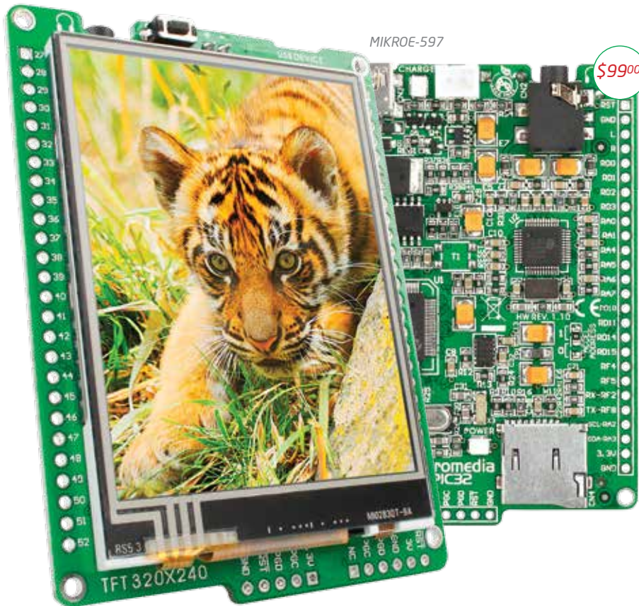
mikromedia for PIC32 (features PIC32MX460F512L)
