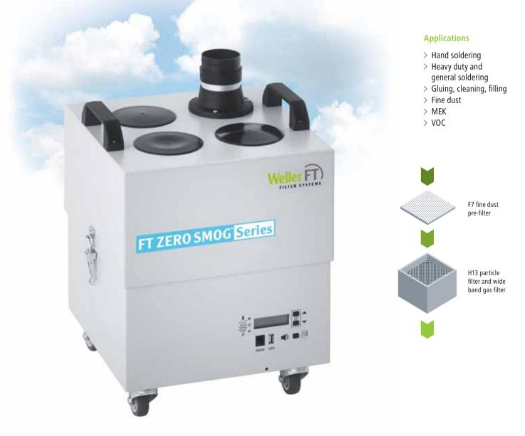
The fume extraction unit Zero Smog<sup>®</sup>4V (ZS4V) is easy to install and operate. The kit is supplied with one flexible hose, one attachment arm with funnel and one bench mount bracket ready for installation at the workplace. A powerful, maintenance-free turbine provides continuous fume extraction at a maximum air extraction rate of 230 m3/h. When setting the Constant Flow Control, the adjustable turbine speed avoids unnecessary waste of power and saves energy.
