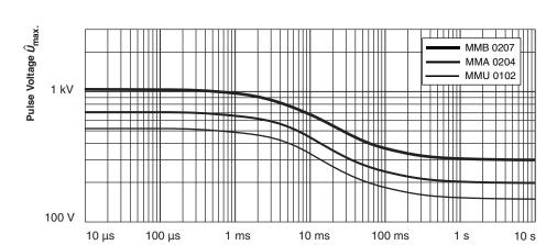
Pulse Duration t; Maximum pulse voltage, single and continuous pulses; applicable if  $\widehat{P} \leq \widehat{P}_{max}$ ; **Pulse Voltage** for permissible resistance change equivalent to 8000 h operation
