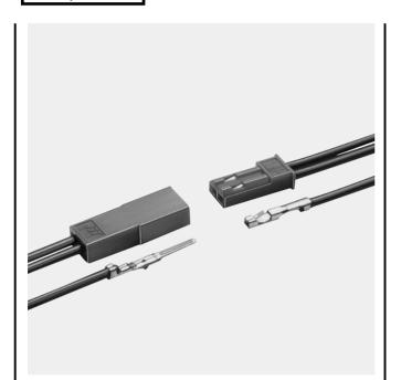
The RCY connector is a compact, 2.5mm pitch wire-to-wire connector for use with a variety of circuits, from signal circuits to power supply circuits, in electrical equipment which is becoming more and more compact. The employment of a free spring contact method ensures stable contact performance, and superb working efficiency of insertion and removal.
