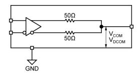
Figure 4b. LVDS Common Mode Measurement
