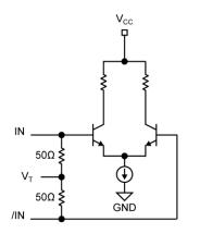
Figure 3. Simplified Differential Input Stage
