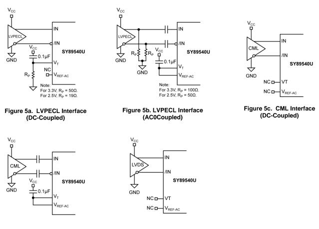
Figure 5d. CML Interface (AC-Coupled)
