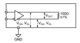
Figure 4a. LVDS Differential Measurement
