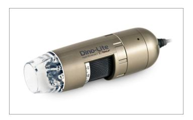
The AM4113TL is a special model with long working distance up to 15 cm at 20x magnification and around 4cm at 90x magnification. The extra working distance makes the TL series an ideal solution for tasks where you need more working distance to the object, for example repair, rework or assembly tasks. The enhanced color sensor provides superior color rendering and improved low light imaging.
