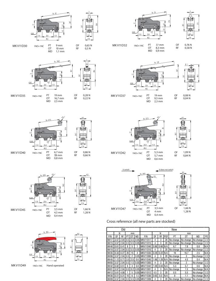
OF= Operating Force (maximum) RF= Releasing Force (minimum) PT= Pre-travel (maximum)
