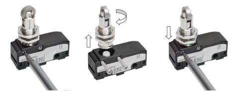
The microswitches have been designed to allow the user to rotate the actuator head (roller plunger types only) by 90° steps and this is possible by removing the holding screws, rotating the head and then refitting the screws back.
