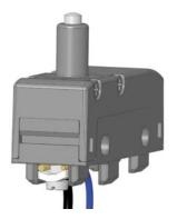
The clamping mechanism of the MK microswitches has been designed to allow for connection of different diameter cables. The clamping plate is designed in such a way to force the cable towards the screw hence achieving the most robust termination possible for all cable sizes within its specification.
