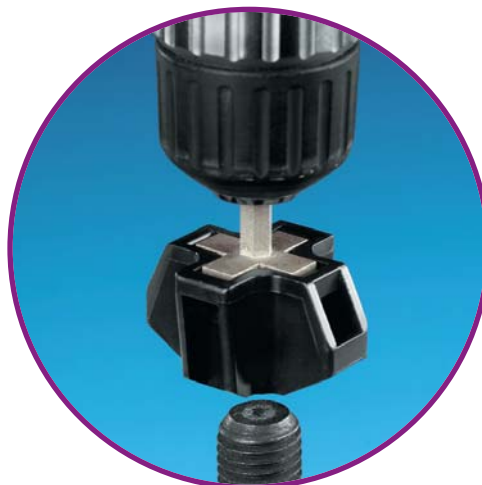
During installation, the custom Stud Mount drill bit application tool ejects itself from mounting base, ensuring proper torque and preventing cracking or breaking of the mount from being overtightened.
