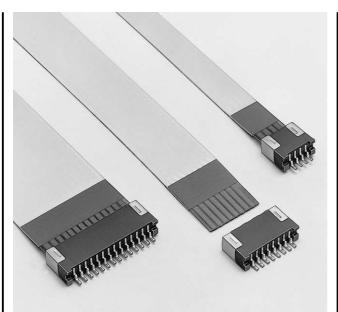
The FMS series connectors are designed for surface mounting (SMT) and to meet the demand for high-density packaging. They are miniature connectors with a height of only 2.8mm (.110"), and can be supplied packaged in embossed tape to facilitate automatic mounting.
