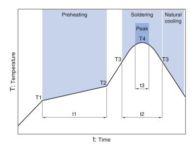
Preheating Soldering Peak Temp. Time Temp. Time Temp. Time T2 T3 T4 t3 250 to 260°C 150°C 180°C 60 to 120s 30 to 60s 230°C 10s max.
