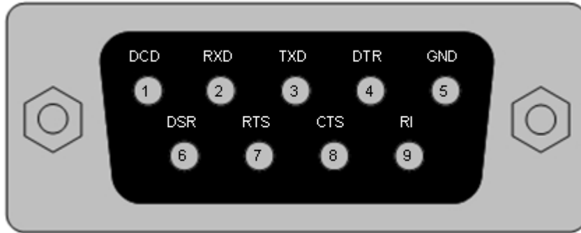
Figure 3-1 RS232 DB9 Pin Out
