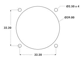
The joystick is mounted from beneath the panel. The gaiter must be passed through the panel cut-out and held in place with the mounting bezel. It is recommended to use No. 2 self tapping countersunk screws, the length of which must be determined subject to the thickness of the panel.
