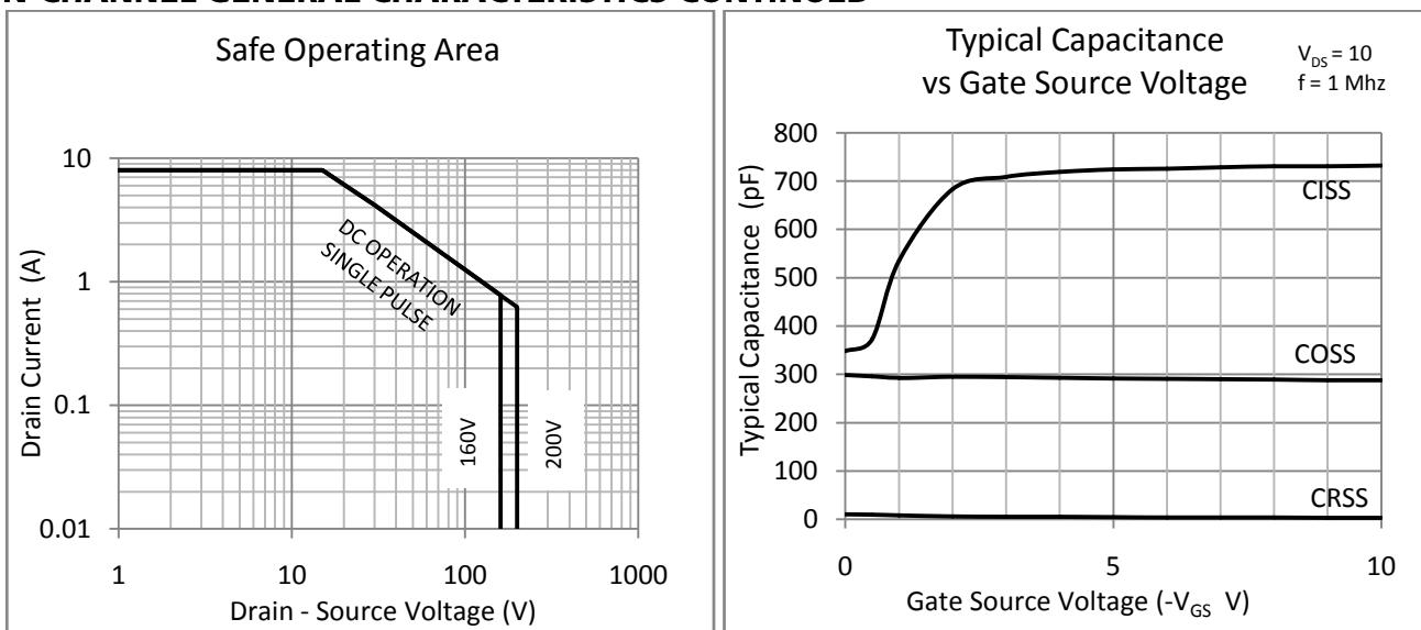
**P-CHANNEL GENERAL CHARACTERISTICS** ( $T_C = 25^\circ\text{C}$  unless otherwise stated)
