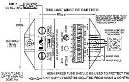
HIGH SPEED FUSE SHOULD BE USED TO PROTECT THE DEVICE UNIT SUPPLY MUST BE ISOLATED FROM MAINS & CONTROL SIGNAL
