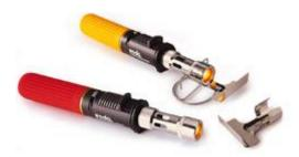
The MJ-950 Ultra-Therm is designed for industrial use where high volume flameless heat is required. Its wide nozzle and high-output long life catalyst provide for infinitely adjustable heat levels in a completely portable tool. Safe to use underhood where vaports may be present. Included deflector attachments makes large heavy-wall shrink tubing a zap to install. Use almost anywhere you would use a corded heat gun but WITHOUT THE EXTENSION CORD!
