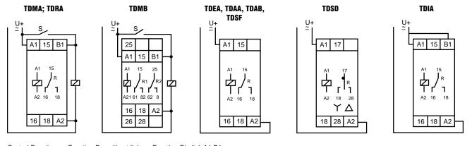
Control Function Function Rp: without link Function Ri: link A1-B1
