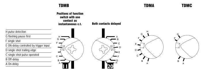
Start function B, C, D, E and H by control contact A1-B1
