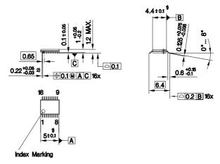
1) Does not include plastic or metal protrusion of 0.15 max. per side 2) Does not include dambar protrusion
