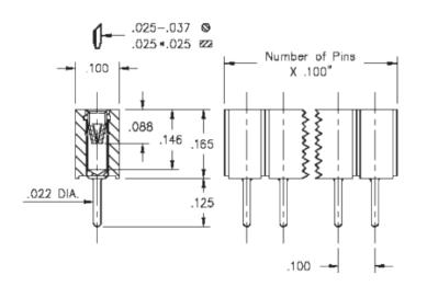
Interconnect Socket Standard Solder Tail Socket Accepts .025"- .037" (0,635 - 0,94 mm)dia leads Single Row Through Hole Plating Code: 43 Shell Plating: 200 µ" Tin (matte finish) over 100 µ" Nickel Inner Contact Plating:
