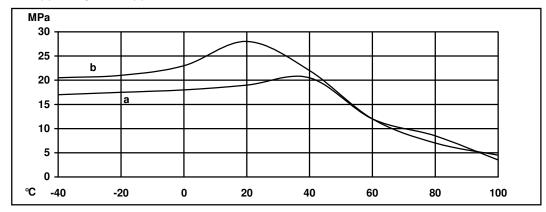
Roller peel test (ISO 4578) (typical average values) - Cure: 16 hours/40°C
