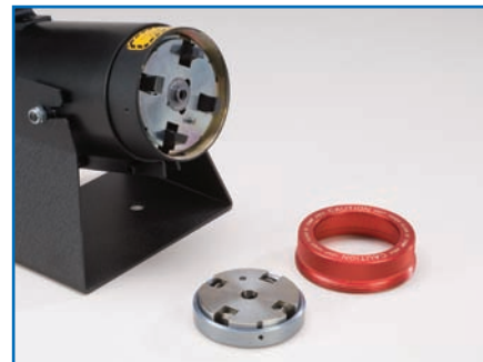
2. Pull off Indenter Die Assembly by hand.
