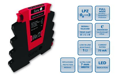
Combined Category D, C, B tested protector (to BS EN 61643) suitable for twisted pair 4-20 mA loop systems with innovative LED protector status indication. For use at boundaries up to LPZ  $0_B$  to protect against flashover (typically the service entrance location) through to LPZ 3 to protect sensitive electronic equipment (e.g. transmitters, monitors, controllers).
