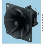
Power Rating Frequency Response Sensitivity (SPL 2.83V/1m) Overall Dimensions (WxH) Cut Out Mounting Depth Weight 225W (4Ω) / 115W (8Ω) 4000Hz - 20000Hz 94dB 85x85mm Ø77mm 60mm 60g
