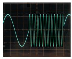
Frequency switching in FSK mode.
