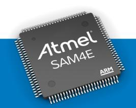
The Atmel® | SMART SAM4E family of microcontrollers (MCUs) delivers a rich set of advanced connectivity peripherals and a floating point unit (FPU). Based on the 32-bit ARM® Cortex®-M4 processor, SAM4E devices operate up to 120MHz and offer up to 1024KB of Flash, 2KB of cache memory and up to 128KB of SRAM. The family further extends a growing Atmel portfolio of ARM processor-based devices.
