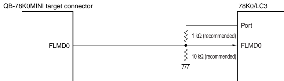
Figure 25-2. Connection of FLMD0 Pin for Self Programming by Means of On-Chip Debugging
