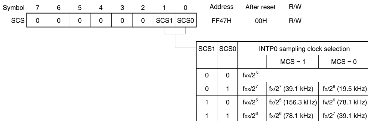
Figure 21-7. Format of Sampling Clock Select Register
