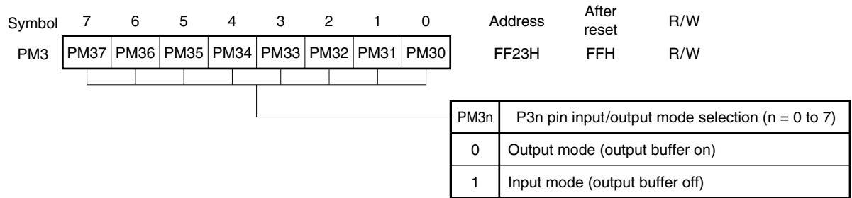
Figure 13-3. Format of Port Mode Register 3
