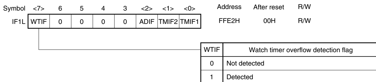
Figure 21-19. Format of Interrupt Request Flag Register 1L
