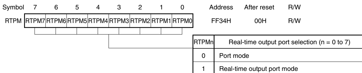
Figure 20-4. Format of Real-Time Output Port Mode Register
