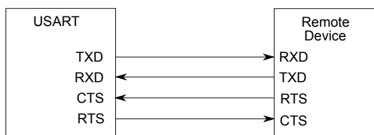
Figure 32-7. Connection with a Remote Device for Hardware Handshaking
