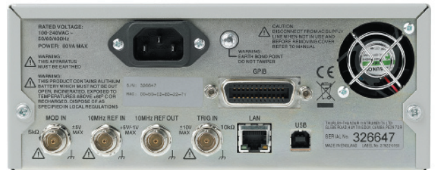
Rear panel mounts the digital interfaces and the rear I/O connectors. (Note: GPIB interface is an option)
