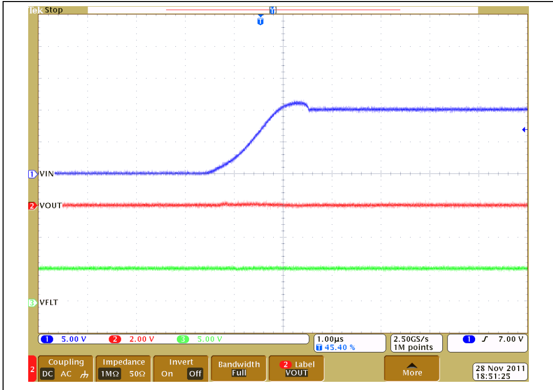
Figure 15. Startup to overvoltage (detail)
