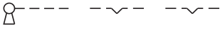
16 Keylock switch actuator 2 positions page 15 | Keylock switch actuator 2 positions, flush mounting page 21
