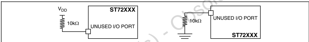
Figure 61. Two typical Applications with unused I/O Pin
