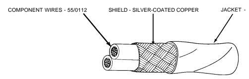
LOW OUTGASSING, RADIATION-CROSSLINKED, MODIFIED ETFE
