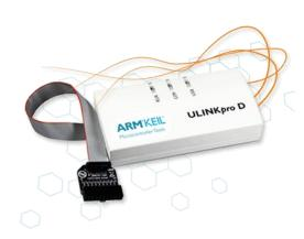
The Keil ULINK*pro* Debug and Trace Unit connects your PC's USB port to your target system (via a JTAG, Cortex Debug, or Cortex Debug+ETM connector). It allows you to program, debug, and analyze your applications using its unique streaming trace technology.
